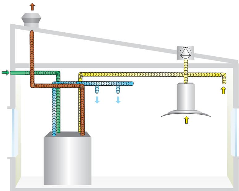
Cooker hood connected to separate roof fan
