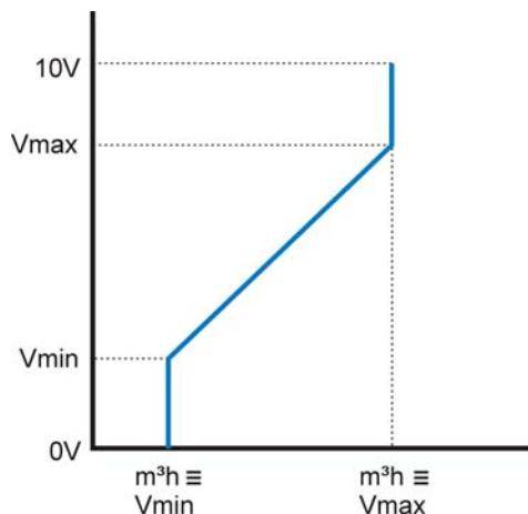
Value  $m^3/h \equiv V_{min}$  can be smaller or greater than  $m^3/h \equiv V_{max}$ .
